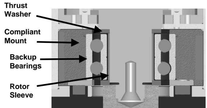
Figure 2. Thrust Backup Bearing Arrangement
