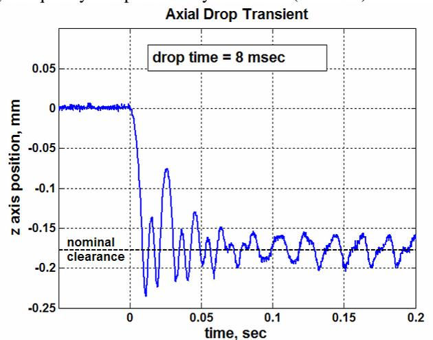
Figure 5. Time history from axial (vertical) position sensors during drop transient at 36,000 rpm.
