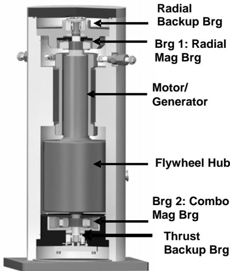
Figure 1. 140kw Flywheel Module
