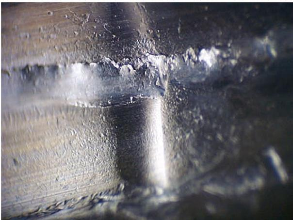
Figure 4. Failed Backup Bearing Inner Race
