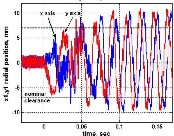
Figure 6. Time history from X & Y Position Sensors during drop transient at 36,000 rpm.
