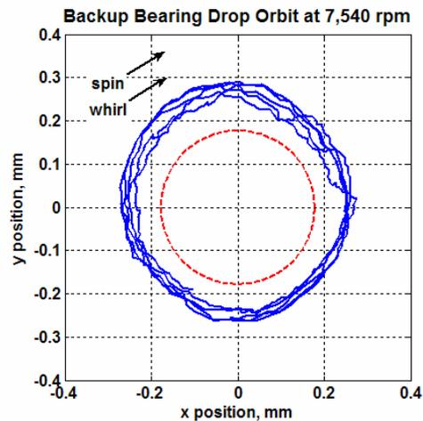
Figure 11. Time History (a) and Orbit (b) from X & Y Position Sensors at 7,540 Rpm
