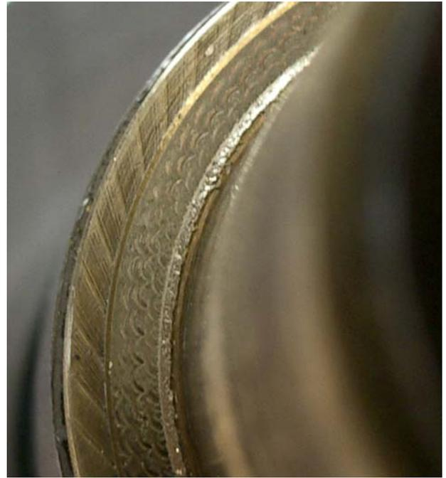
**Figure 3. Wear Track on Rotor Thrust Washer**
