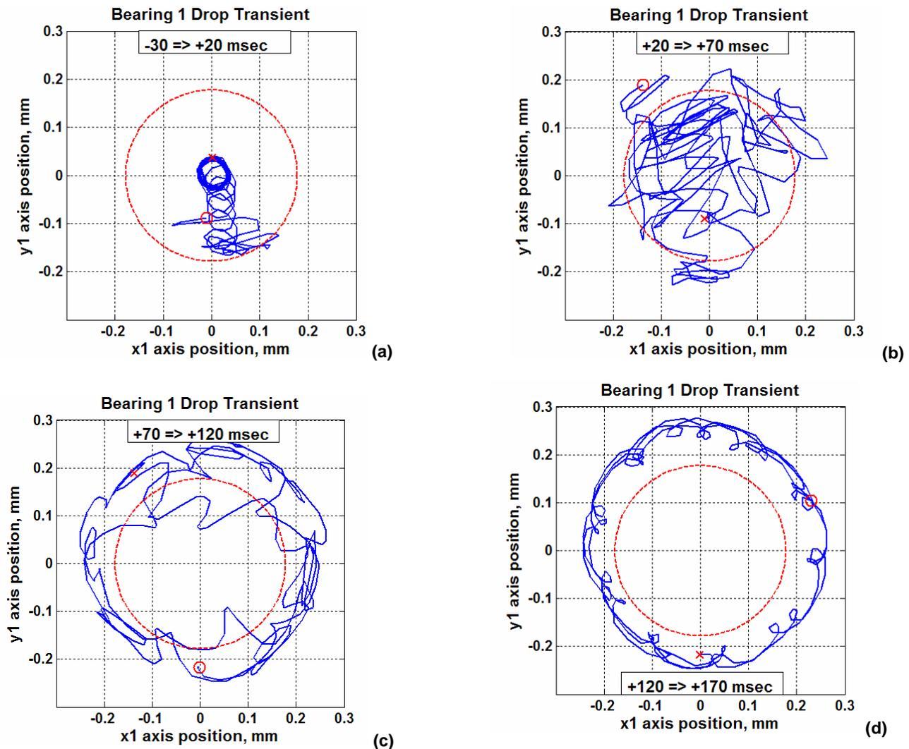
Figure 7. Orbit plot X & Y Position Sensors during drop transient at 36,000 Rpm: (a) -30 -> +20 msec, (b) +20 -> +70 msec, (c) +70 -> +120 msec, (d) +120 -> +170 msec,
