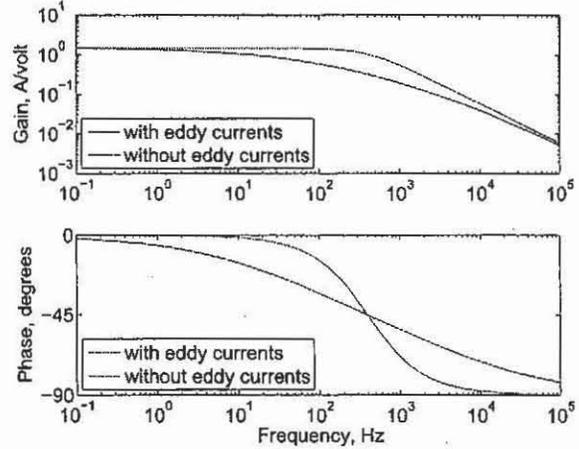
Fig. 4. Bode diagrams of  $G_a(s)$  (no eddy currents in the model) and  $G_a(s, c')$  (includes eddy currents in the model).
