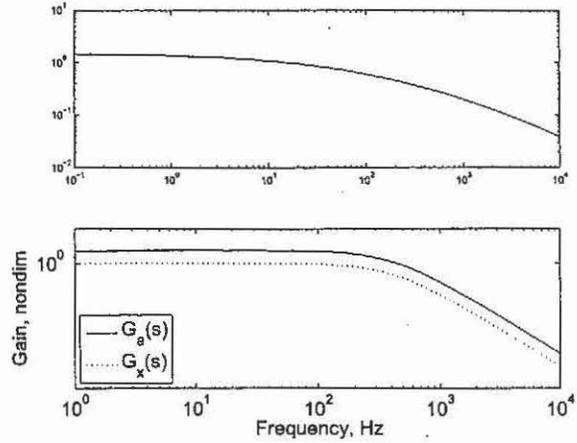
Fig. 2. Gain plots of  $G_a(s)$  and  $G_x(s)$  for the thrust example without eddy currents.
