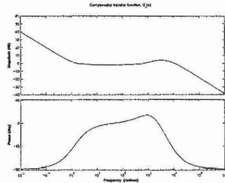
Fig. 3. Thrust bearing compensator Bode plot.
