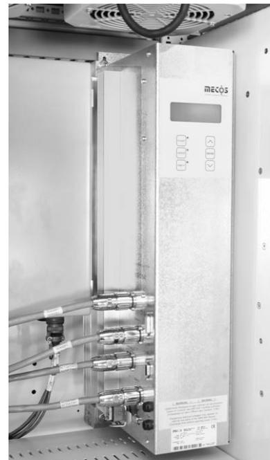
Figure 6. Production controller mounted in flywheel cabinet.
