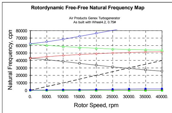
FIGURE 5. Natural frequency map with wheel W1.
