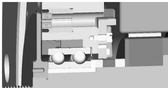
FIGURE 2. Cross-section showing radial/thrust backup bearing.
