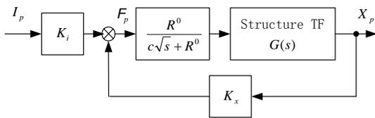
Fig. 6: Block Diagram for a Solid Actuator Operated in the Current Mode
