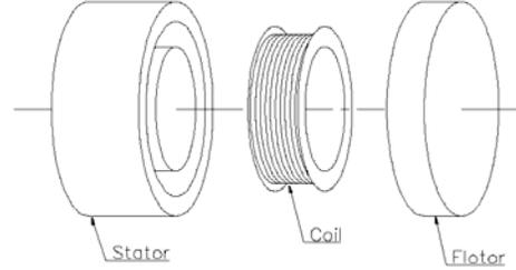
Fig. 2: Exploded View of A Solid Cylindrical Actuator
