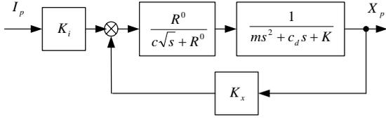
Fig. 9: Block Diagram of the Experimental Test Rig
