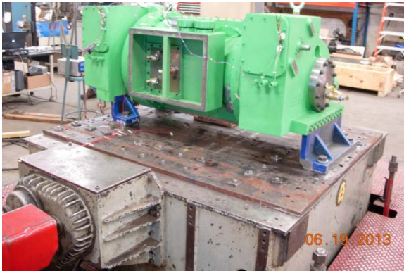
Figure 1. HES-C Compressor Mounted on the Shaker Table.
