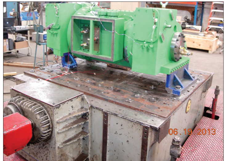
FIGURE 6. Compressor on shaker table for stand-alone tests [3]
