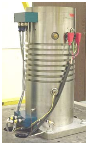
Figure 1. Energy Storage Flywheel
