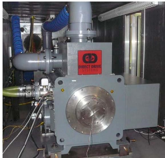
Figure 1. 1MW 15kRPM PM Motor on Magnetic Bearings.
