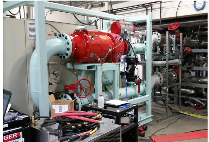
Figure 9. ORC under test at the Calnetix ORC Test Facility.
