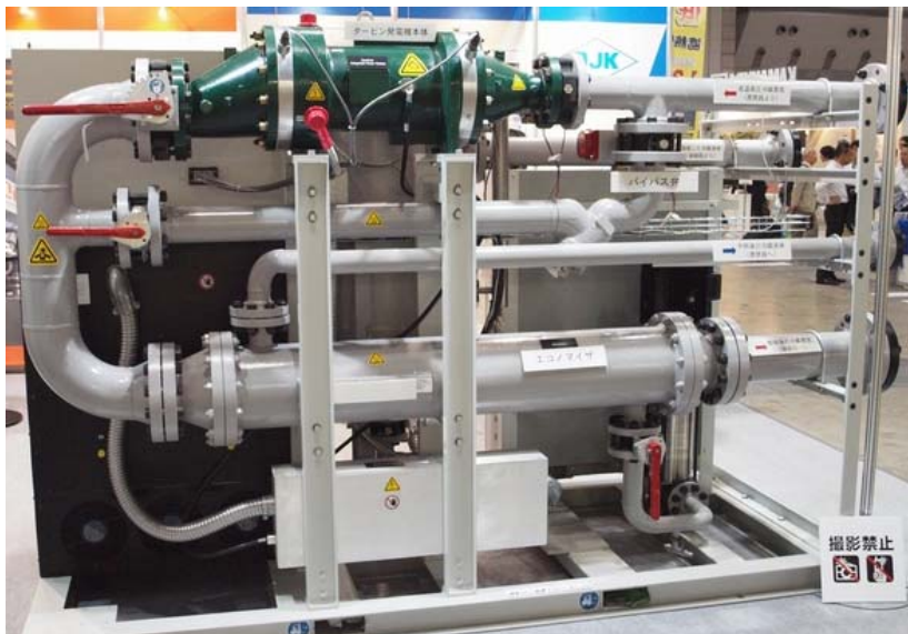
Fig. 3 Binary generator "Thermapower 125MT"
