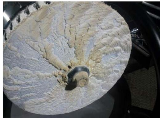
Fig. 2. Atomizer wheel with uneven buildup.
